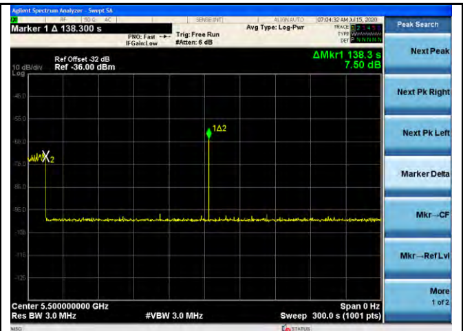
Radar at end of CAC - 5500MHz
