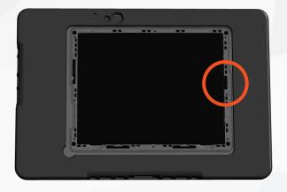
**4.** Enter the Micro SIM card into the slot in the center of the right side. Make sure you have the Micro SIM card in the correct direction (chip facing down).
