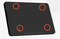
3. Then replace the 4 corner hex screws of the battery cover using the provided hex tool. The recommended torque for the screw is 10-12Ncm.
