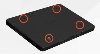
**1.** Remove the 4 hex screws from the corners of the battery cover using the provided hex tool.
