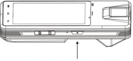
Long press power button two seconds to do On/Off operation
