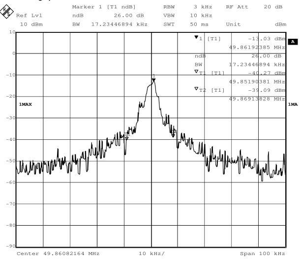
26dB bandwidth lower frequency: 49.85190381 MHz 26dB bandwidth upper frequency: 49.86913828 MHz
