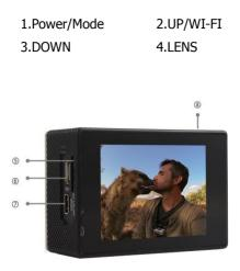
5.TF card slot 7.HDMI 6.USB slot 8.OK
