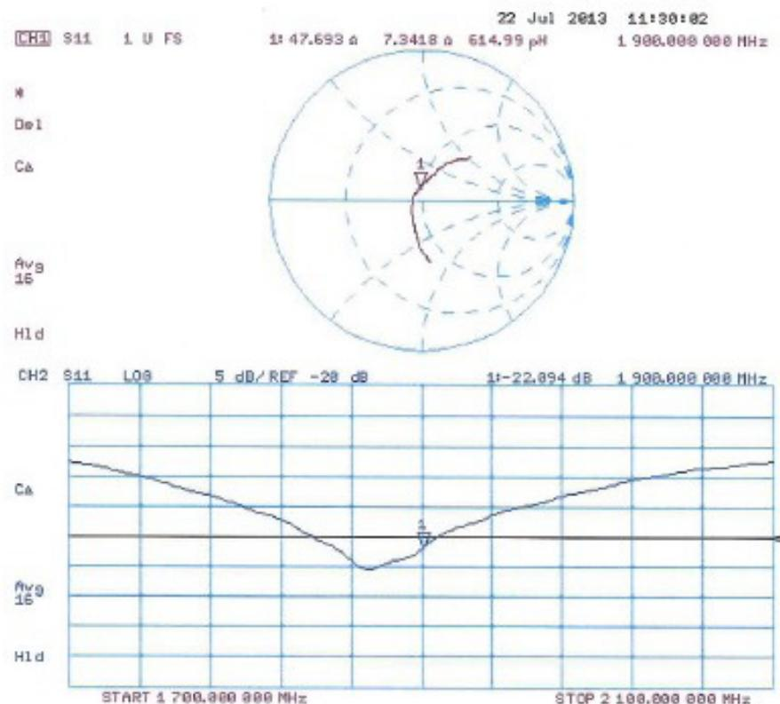
**D1900V2, Serial No.5d136 Extended Dipole Calibrations**
