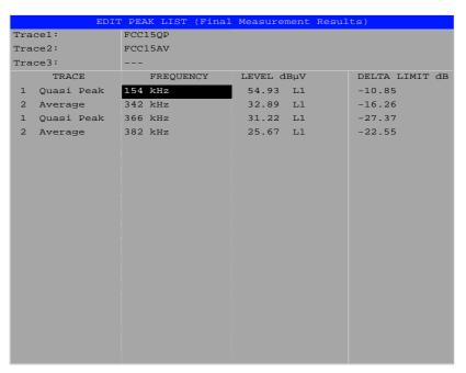
Tested Wire: Neutral Operation Mode: Operate at 2440MHz Continues transmit
