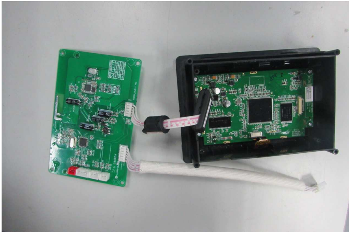
The control circuit box view (Include control circuit and Display circuit)
