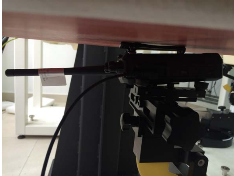
Body-worn, the front of the EUT towards ground with A1, B2, BC2, C1 and D1 (The distance was 0mm)
