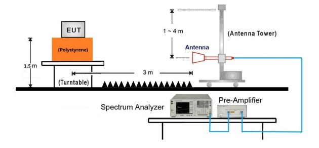
18GHz ~25GHz Test Setup:
