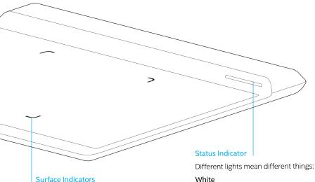
These corners indicate the active charging area, make sure smaller devices are placed within them with the screens facing up.
