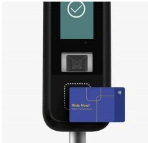
Passing the NFC card in front of the NFC antenna
