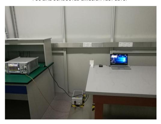
FCC RADIATED EMISSION TEST SETUP
