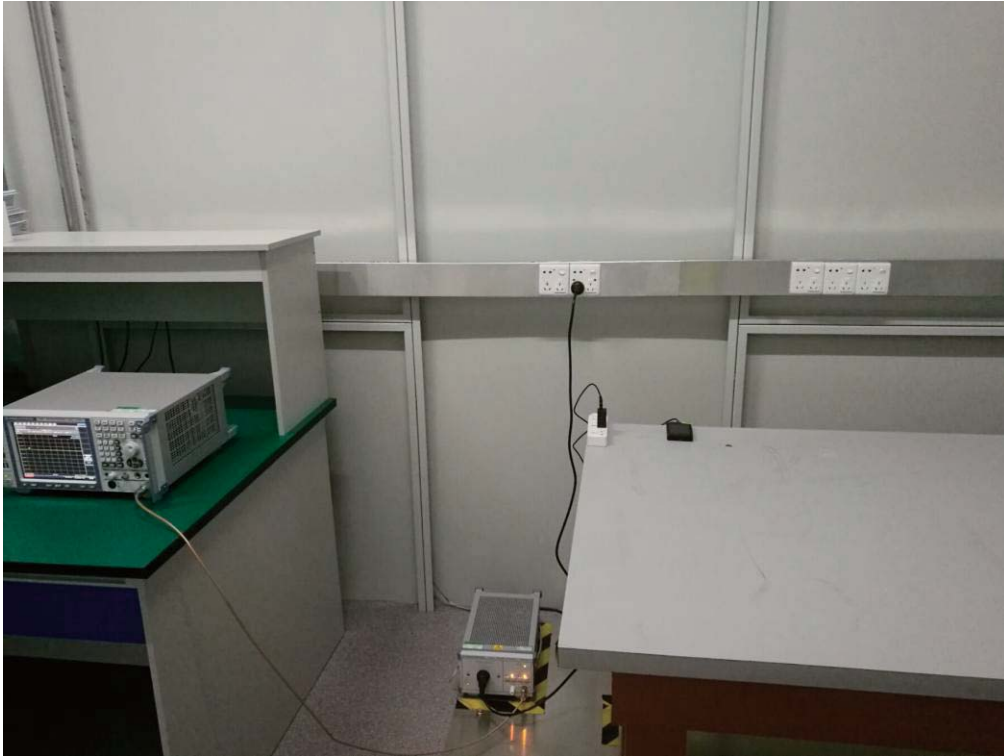
RADIATED EMISSION TEST SETUP
