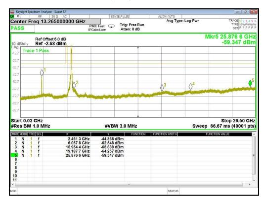
Note:1.The emission levels of other frequencies were less than 20dB margin against the limit. 2.Max Value (dBm) is added antenna gain.
