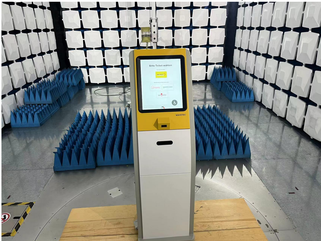
Above 1GHz for radiated emission test setup
