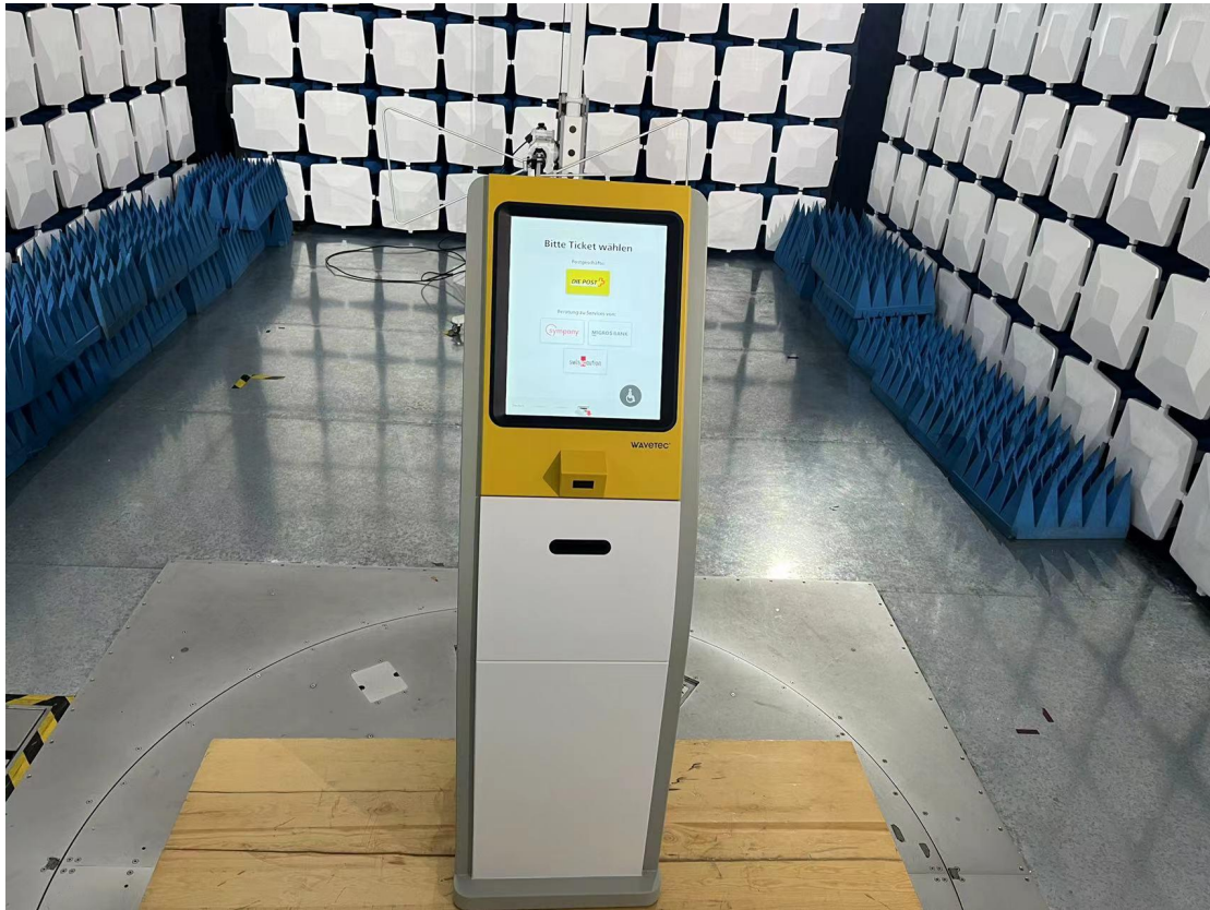
Blow 1GHz for radiated emission test setup
