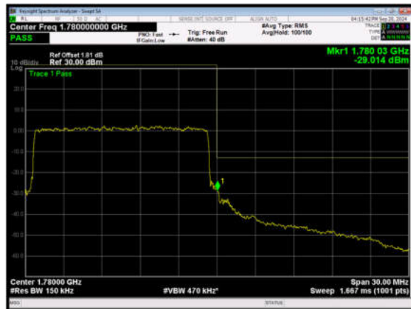
LTE Band 66 QPSK 20MHz CH-High, 1 RB
