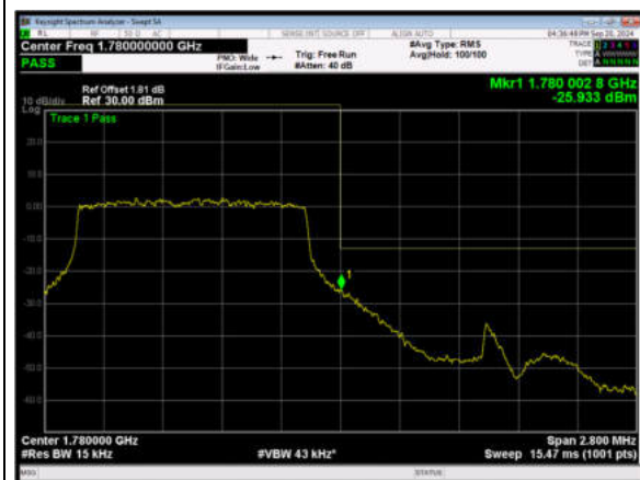
LTE Band 66 16QAM 3MHz CH-High, 1 RB
