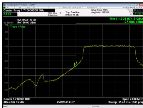
LTE Band 66 16QAM 3MHz CH-Low, 1 RB
