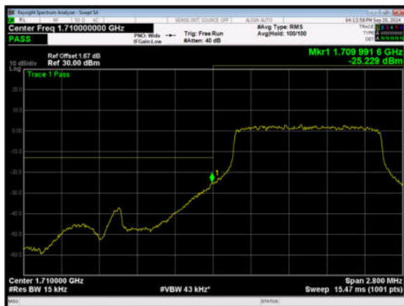
LTE Band 66 QPSK 3MHz CH-Low, 1 RB
