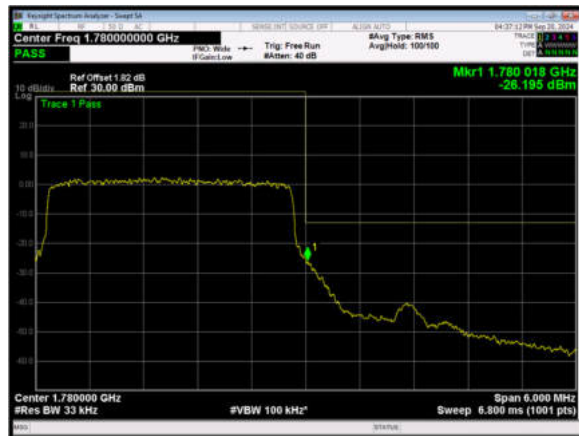
LTE Band 66 16QAM 5MHz CH-High, 1 RB
