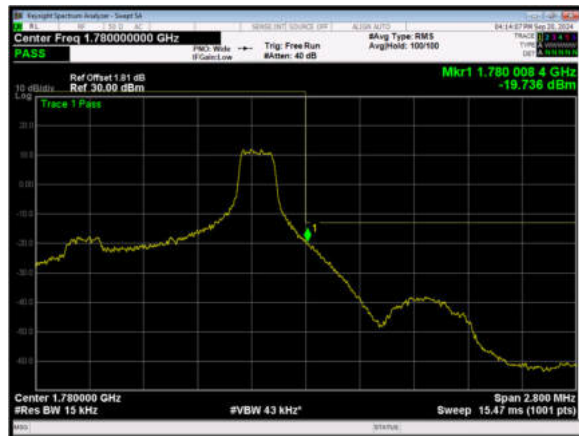
LTE Band 66 QPSK 1.4MHz CH-High, 100%RB
