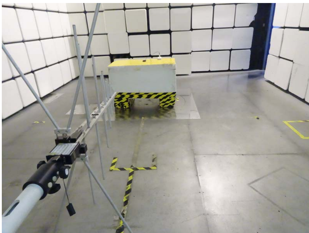
Picture 1 Radiated Emission Test Setup
