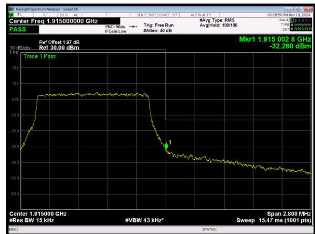
LTE Band25 16QAM BW=1.4MHz Channel=26683 RB Size=6 Position=#0
