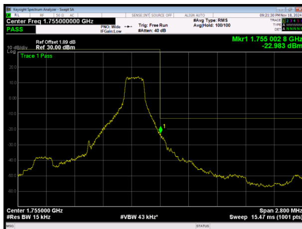
LTE Band4 QPSK BW=1.4MHz Channel=20393 RB Size=1 Position=#Max
