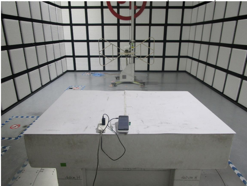
RADIATED RF MEASUREMENT SETUP (30MHz~1GHz)
