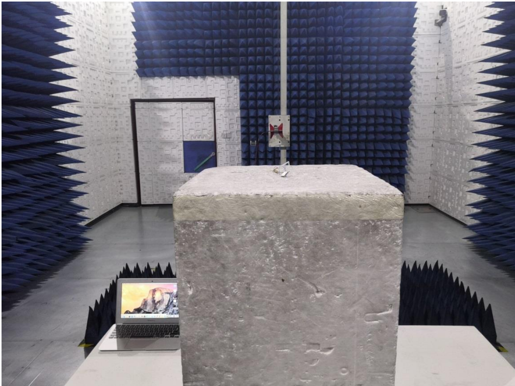
RADIATED EMISSION TEST SETUP ABOVE 1GHZ
