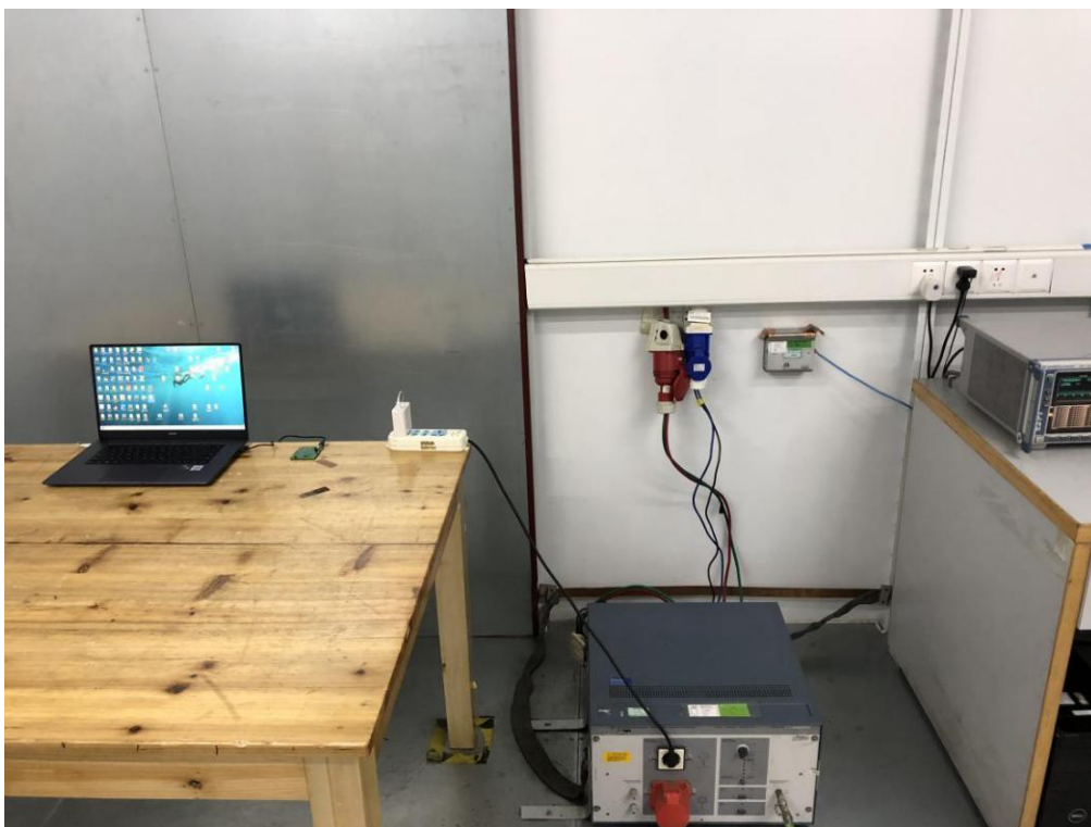
LINE CONDUCTED EMISSION TEST SETUP
