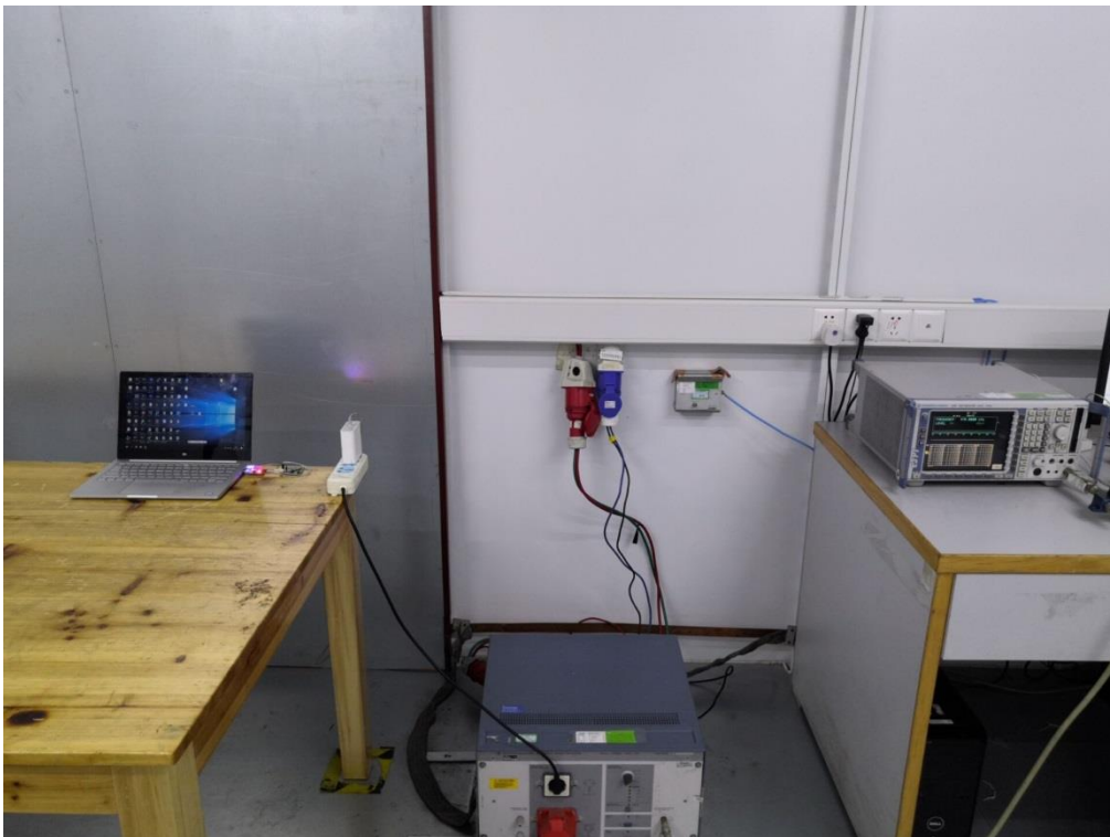
CONDUCTED EMISSION TEST SETUP
