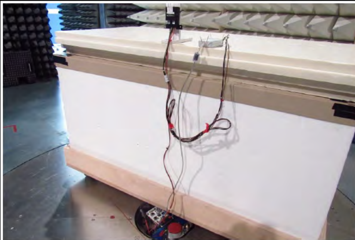
EUT Setup below 1 GHz
