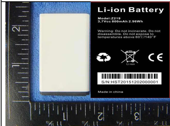
Battery - Front View
