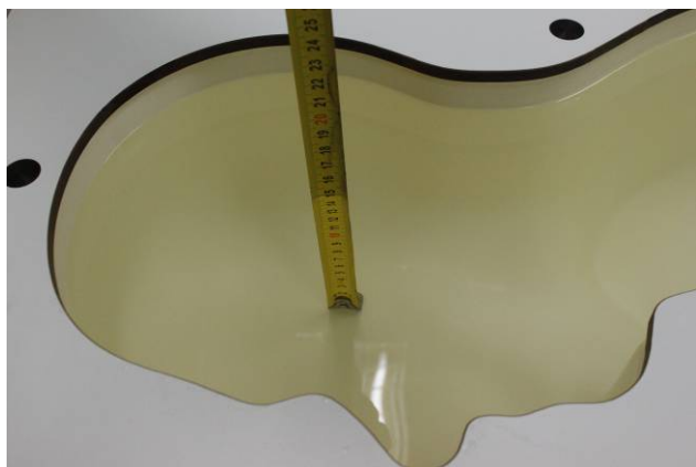
Liquid depth in the head Phantom (1900 MHz 15cm depth)
