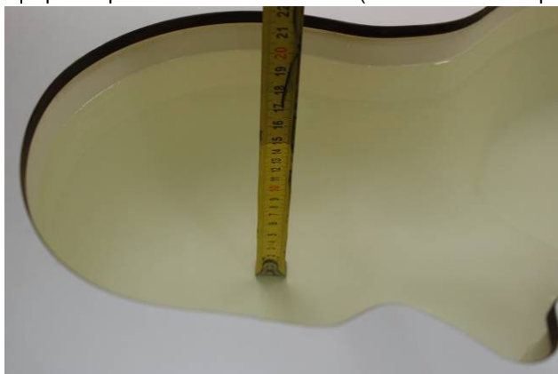
Liquid depth in the head Phantom (1900 MHz 15cm depth)
