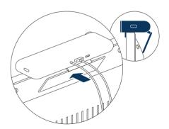
Remove plastic battery tab on the back of remote control.
