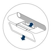
To make sure Portal TV is secure, press back clip firmly against the back of your TV.
