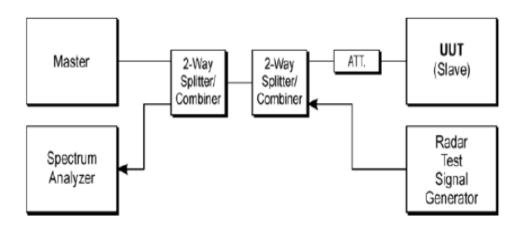
**Radiated Test Setup**
