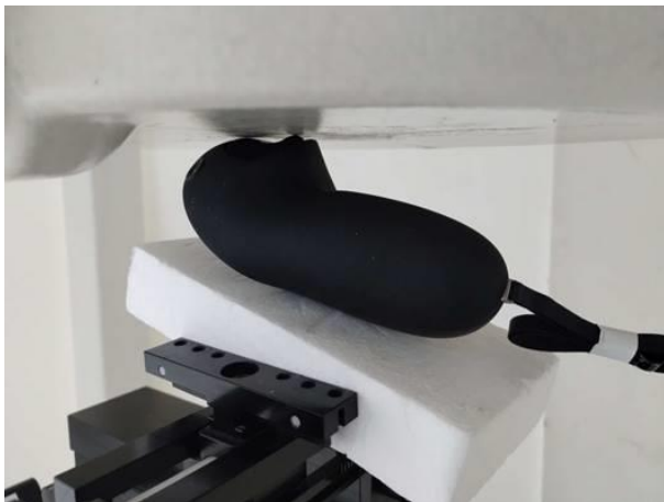
Right Hand Position 2, Test Separation 0 mm
