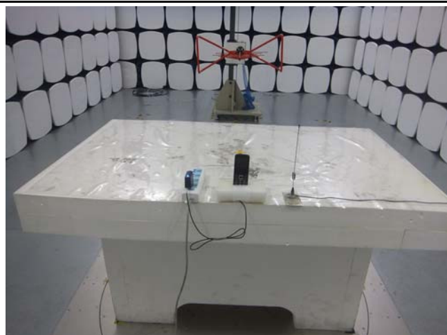
Conducted Emissions Test Setup Front View
