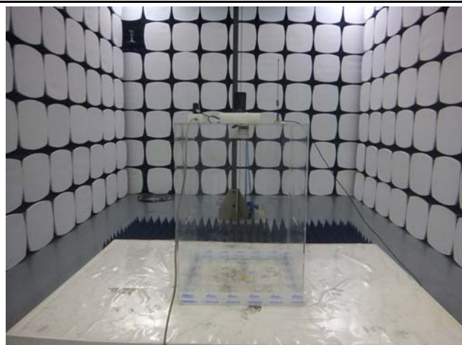
Radiated Spurious Emissions Test Setup Above 1GHz
