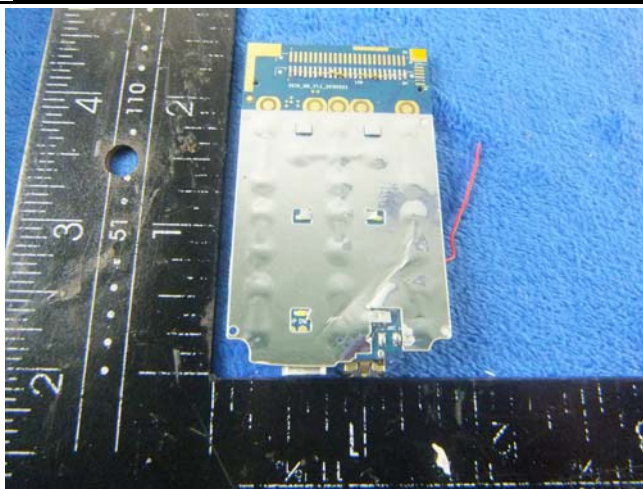
Mainboard with Shielding - Rear View
