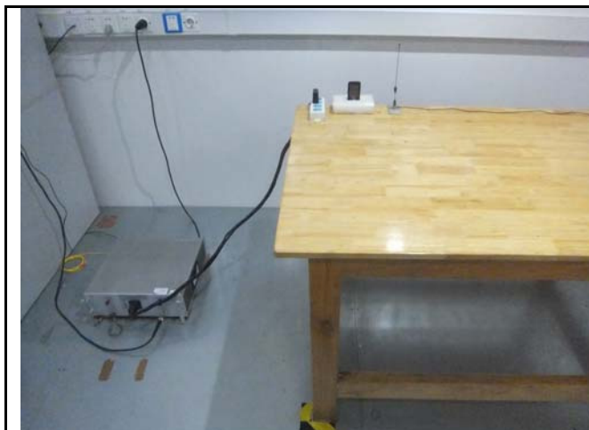
Conducted Emissions Test Setup Front View
