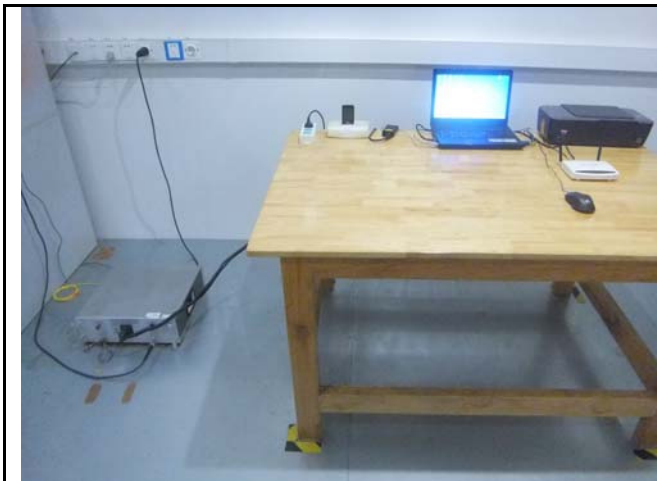
Conducted Emissions Test Setup – Front View
