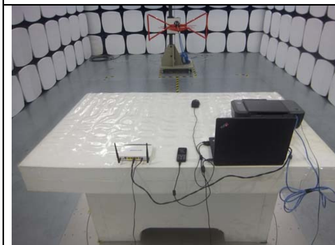
Radiated Emissions Test Setup Below 1GHz
