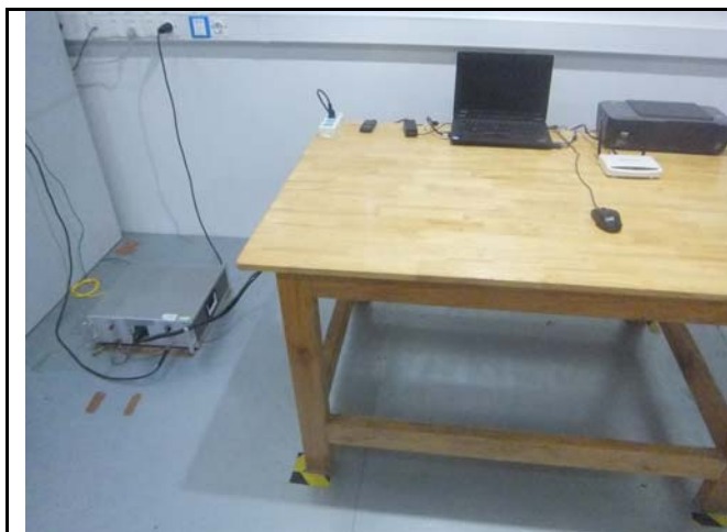
Conducted Emissions Test Setup – Front View
