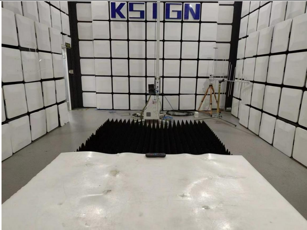
Radiated emissions (Above 1GHz)
