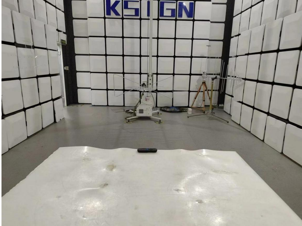
Radiated emissions (Below 1GHz)
