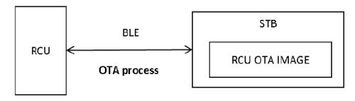
From diagram above, the STB can transfer the RCU firmware by the BLE link.
