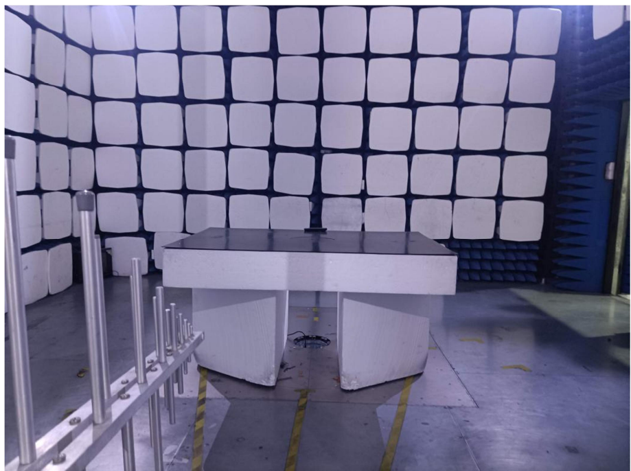
Radiation Emission Test Setup (30MHz to 1GHz)
