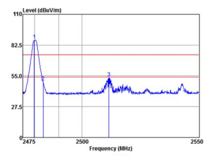
Mode:a; Polarization:Horizontal; Modulation:GFSK; ; Channel:High
