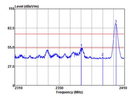
Mode:a; Polarization:Horizontal; Modulation:GFSK; ; Channel:Low
