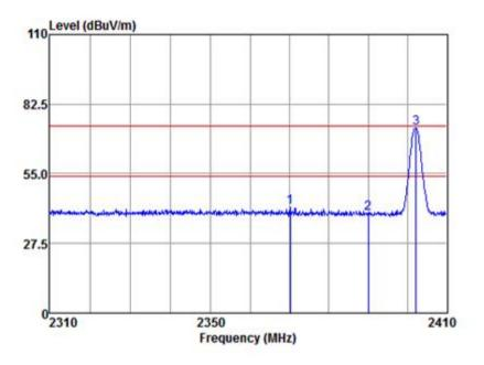
Mode:a; Polarization:Vertical; Modulation:GFSK; ; Channel:Low
