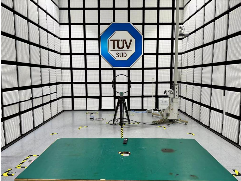
Radiated Emission Setup 9kHz ~ 30MHz
