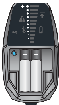
Figure 17. Battery compartment and battery placement
