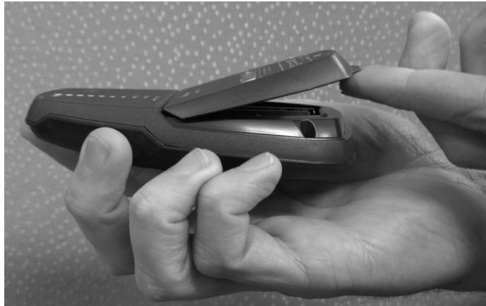
Figure 16. Removing the battery compartment cover
