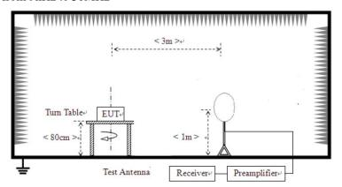
For radiated emissions from 30MHz to1GHz
