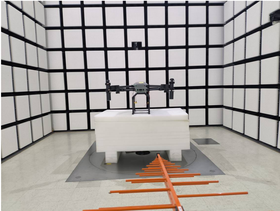
Radiated Emission Above 1GHz View 1-18G
