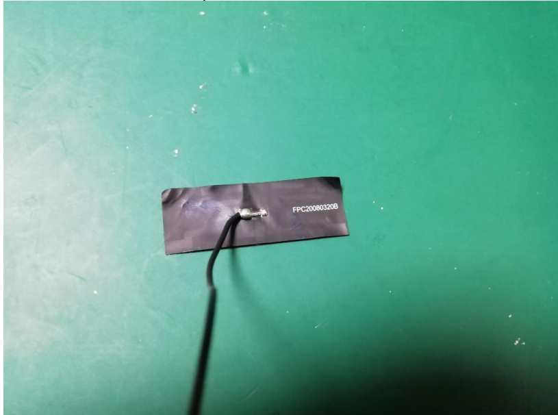
close-up of the 5.1G&5.8G WiFi antenna photo
