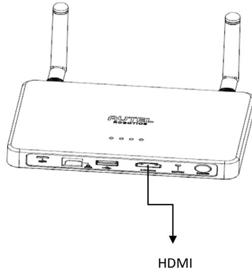
△ Warning: the Live Deck supports connecting the HDMI, Ethernet port and USB port to Android devices at the same time. When the USB port is connected to an iOS devices, the HDMI and Ethernet port will not display image.
