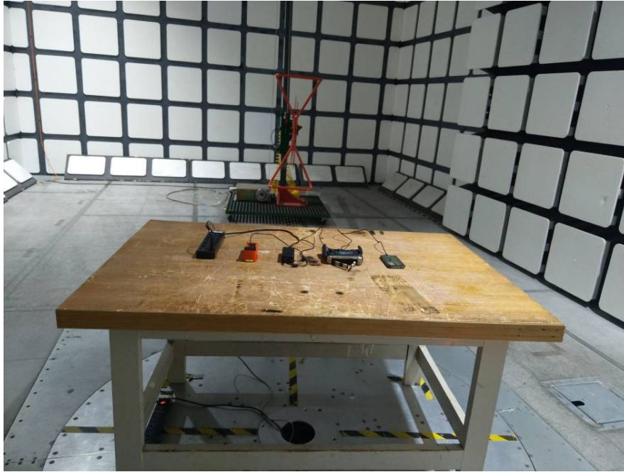
Radiated Emissions View (Below 1 GHz)
