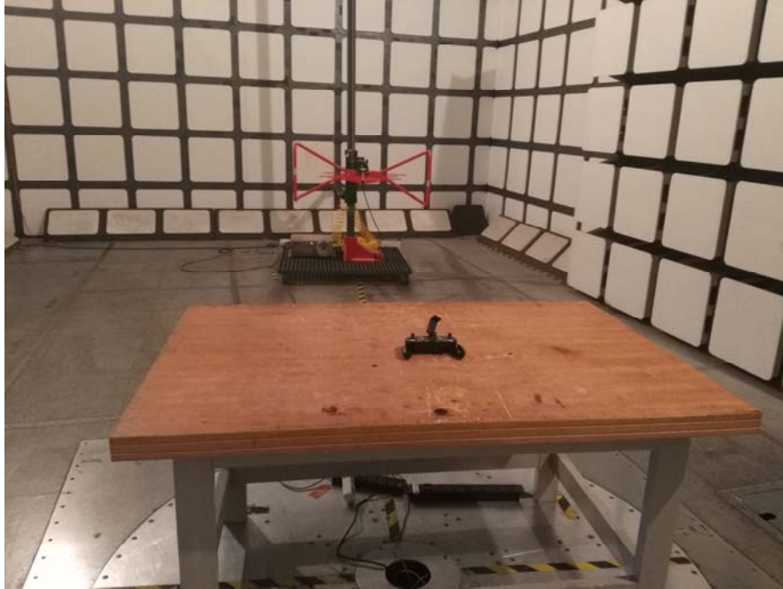
Radiated Emissions View (Below 1 GHz)
