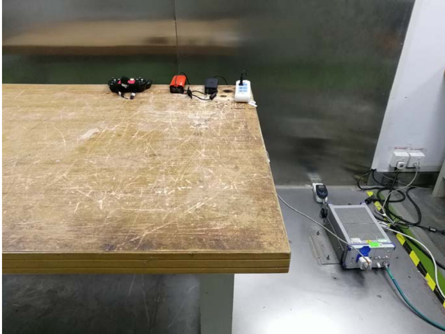
Conducted Emissions - Front View
