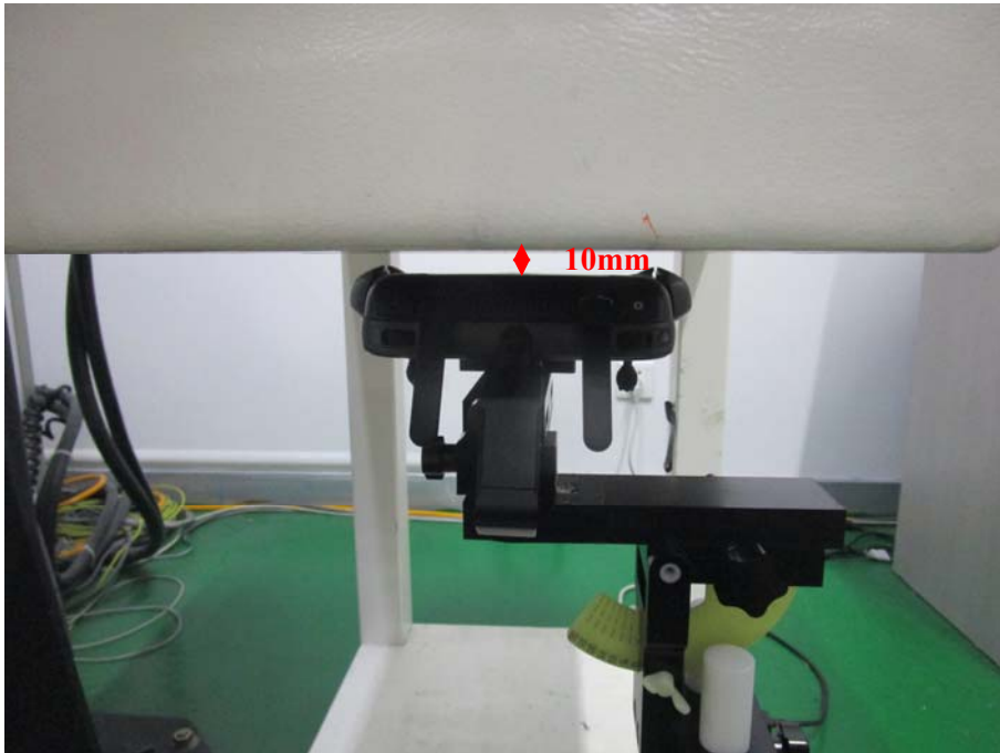
Test Position_Back Antenna Fold (10mm)
