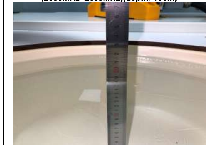
Fig. 9.8 Photo of Liquid Height for Body SAR (5200MHz~5800MHz) (depth>15cm)
