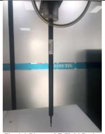
Fig. 8.2 Photo of E-Field Probe
