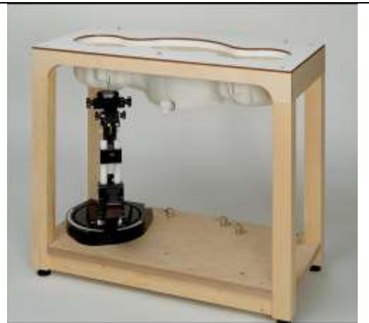
Fig. 8.7 Photo of SAM Twin Phantom
